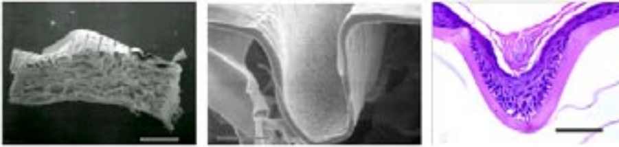
Figure 7. Microfabricated basement membrane analogue. Left panel shows microfabricated basement membrane analogue integrated onto a dermal equivalent. Middle panel shows the detail of the microfabricated membrane at high magnification. The thickness of the membrane is about 10 to 20 \mu\text{m} and the height is 300 \mu\text{m} . Right panel shows the skin equivalent after keratinocytes are grown on the microfabricated membrane and differentiated by bringing to the air-liquid interface during culture.
